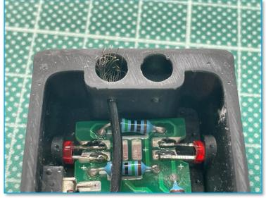
TIP: It is best to insert all magnets with the same polarity. Remember later when fitting magnets to the upper clip housing to orient the correct polarity so they attract, not repel, those fitted to the clip.
