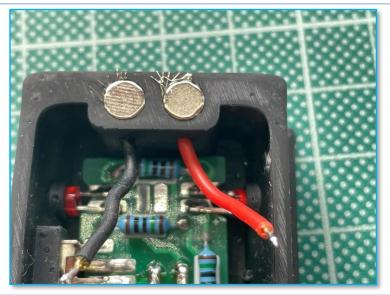
Next you need to solder the wires to the PCB pads.
