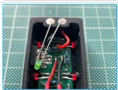
**Use the same technique**, above, when connecting the white figure '8' wire to the upper clip holder. This white wire will route up to the screwdriver/sight rod to power the green LEDs.
