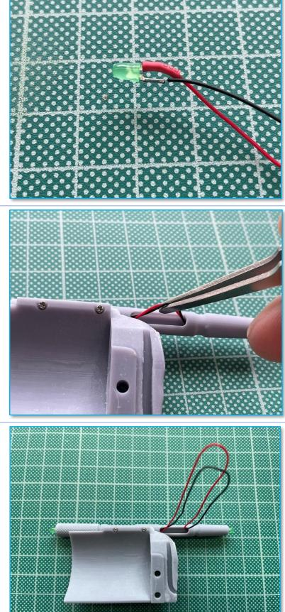
Slide the LEDs into the ends of the sight. Note that there is a correct orientation as the sight has a wider part to accommodate the LED leads.
