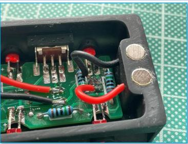
Test the connections to the magnets by holding a green LED onto the magnets.
