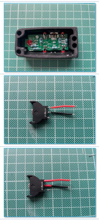
Now solder the wires to the pads on the PCB marked 'BATT'.
